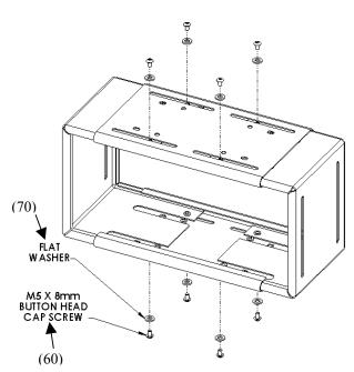
Figure 3. Attach Center Plates and Side Plates
